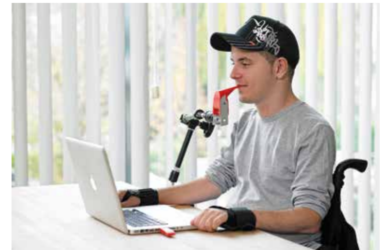
One of the Innovative Practices 2016 from Austria: IntegraMouse is a wireless computer mouse that can be operated with the human mouth for people who are unable to use their hands and fingers.
