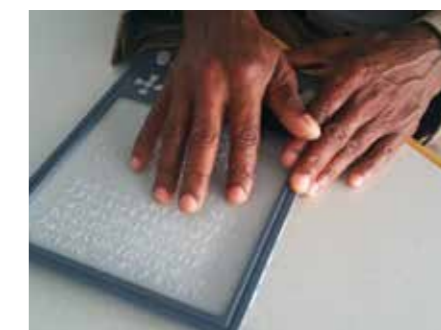
The BLITAB-Tablet generates lines in Braille instead of an LCD screen. It is currently tested by thousands of students.
