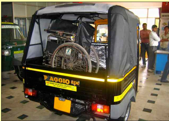
Folded wheelchair in auto-rickshaw at test session. - Photo by AEI
