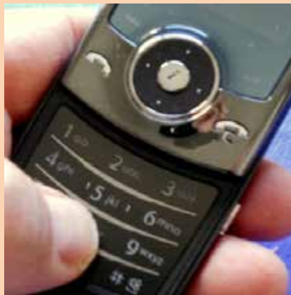
Figure 1.4: Samsung phone with elevated dots on key #5
